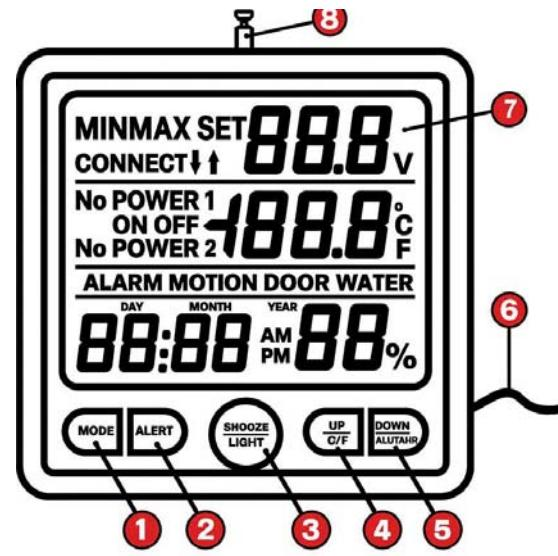
4. **Units / Increase Button (°C/°F)** – This button toggles the temperature units between **Celsius and Fahrenheit** on the display. In Settings Mode, it functions as the “**increase**” button to raise a selected value or scroll up through options.
